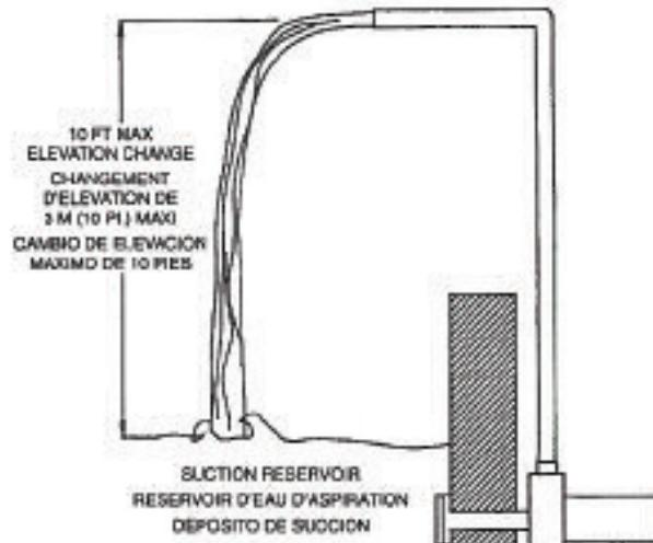
NOTE - SUCTION FITTINGS MUST CONFORM TO ASME/ANSI A112.19.8 M STANDARDS. USE DOUBLE SUCTION FITTINGS.
